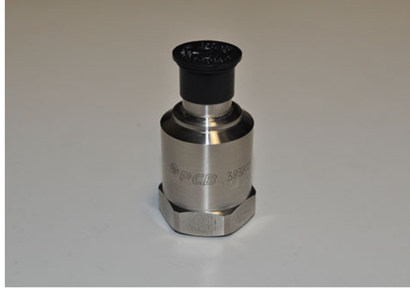
Fig. 3.1 IEPE accelerometers (by PCB Piezotronics Inc.)
