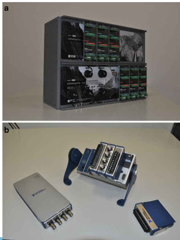
Fig. 3.6 Dynamic data acquisition system by Kinemetrix Inc. (a) and programmable hardware by National Instruments™ (b)
